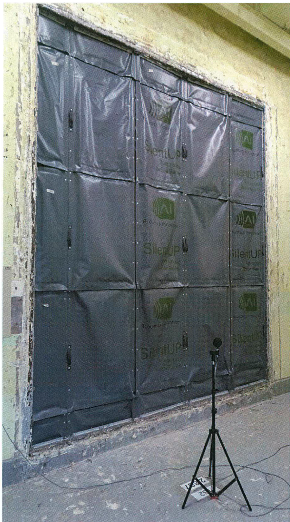
Measurement set-up (Source room)
