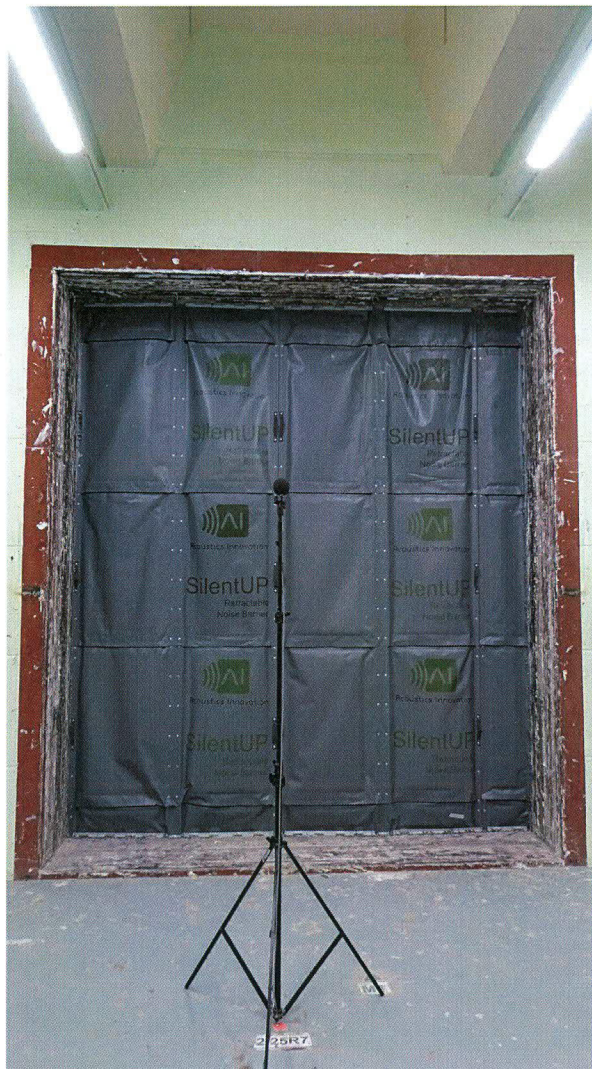
Measurement set-up (Receiving room)
